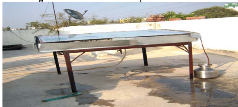
Fig. 1b- Black granite simple basin solar still photograph as mentioned in text
